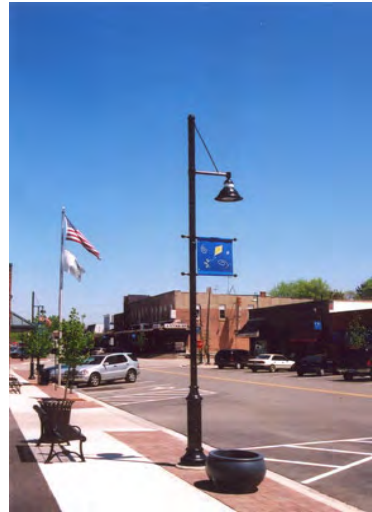
New lighting standards today can be fitted with fixtures that point light downward to minimize spillage.
