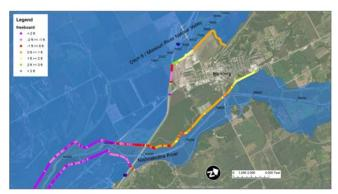
Figure 3.3-10. Estimated freeboard along Nishnabotna River near Hamburg, Iowa. No overtopping allowed.
