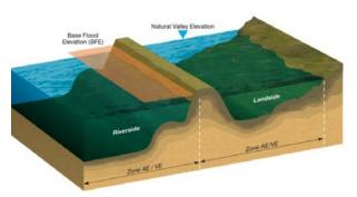
Figure 3.2-3. Cross section of a reach modeled using Natural Valley Procedure.
