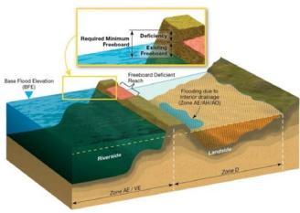
Figure 3.2-6. Cross section of a reach modeled using Freeboard Deficient Procedure.
