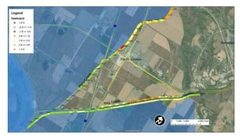
Figure 3.3-17. Estimated freeboard along Pony and Keg creeks near Pacific Junction, Iowa. No overtopping allowed.
