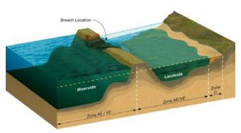
Figure 3.2-4. Cross section of a reach modeled using Structural Based Inundation Procedure.
