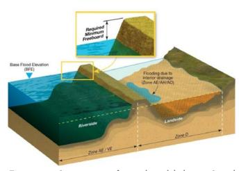
Figure 3.2-7. Cross section of a reach modeled using Sound Levee Procedure.
