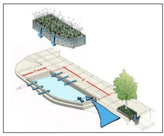
Diagram of how a stormwater bumpout works
