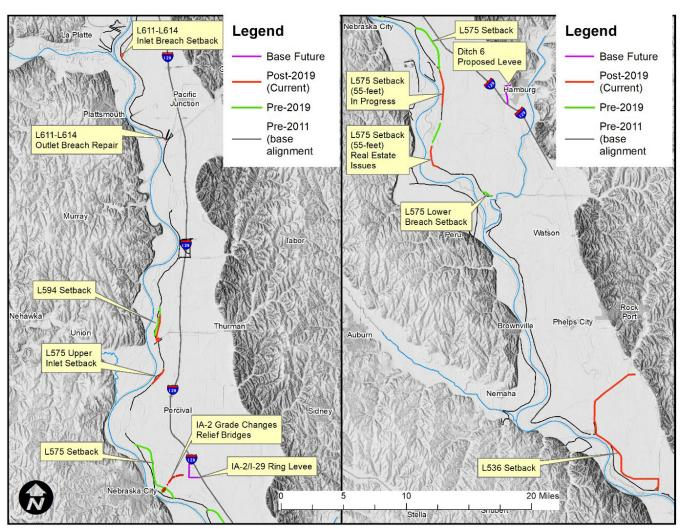
Figure 3.3-3. Levee alignment configurations used in developing model geometries. These include alignments in place during the 2011 and 2019 flood events, levee improvements following the 2019 flood (current conditions), and near future levee changes (base future conditions).
