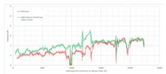
Figure 3.3-23. Estimated freeboard along Pony Creek for the left and right levees.
