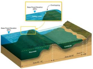
Figure 3.2-5. Cross section of a reach modeled using Overtopping Procedure.
