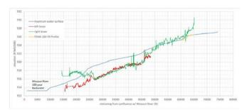
Figure 3.3-11. Water surface elevation profile of the Nishnabotna River shown with left and right top of levee elevations.
