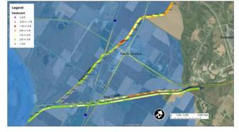
Figure 3.3.3-19. Depiction of inundation behind the levees if Pony Creek is overtopped at lowest freeboard location.
