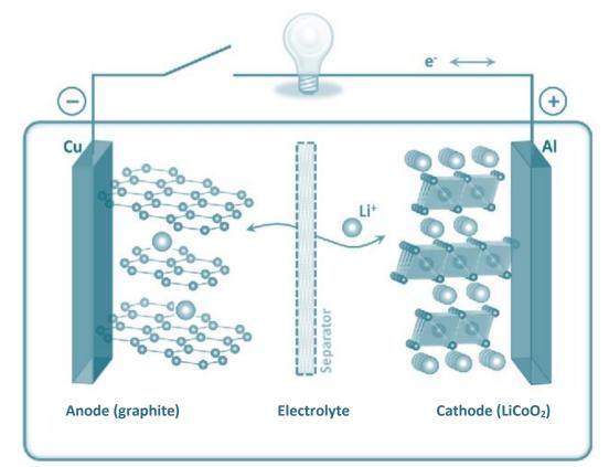
Figure 1. Lithium-ion charging and discharging mechanics
