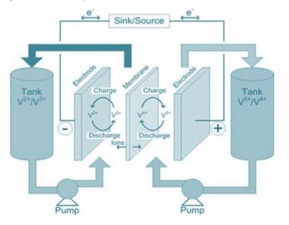
Figure 2. Flow battery schematic
