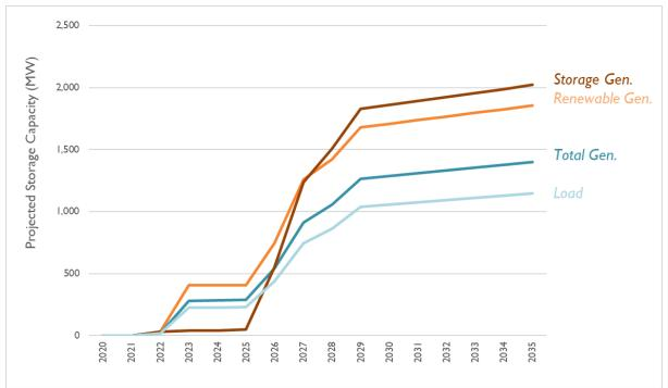
Figure 10. Estimated utility-scale storage capacity projections for each ratio approach from the Colorado study
