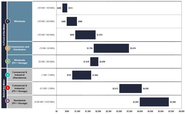
Figure 8. Capital costs comparison (nameplate capacity) of battery storage systems by application (\$/kW)
