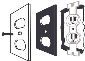
Install foam gaskets between electrical outlets or switches and their coverplates. Plastic plugs—such as "child safety" inserts—also will prevent air from entering your home.
