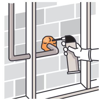
Expanding foam sealant works well for sealing gaps more than 1/4-inch wide.
