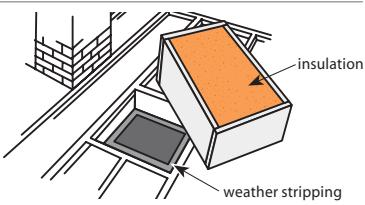
If you have an attic hatch, make sure it fits tightly and is backed by insulation. Do this by weather-stripping the edges of the access hole and building a simple wood box to hold insulation on the backside of the hatch. As an alternative, purchase an insulated hatch cover.
