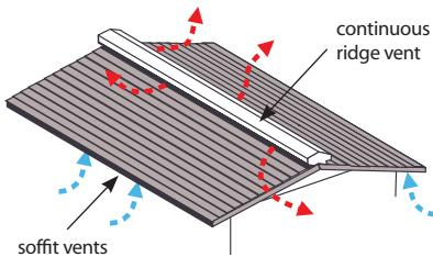
If you're reroofing or building a new home, a continuous ridge vent combined with soffit vents offers optimal attic ventilation. In this illustration, blue arrows indicate outside air flowing into the attic and red arrows show attic air flowing out.
