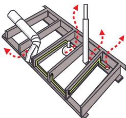
Recessed lights, wiring, plumbing and other openings in insulated ceilings and walls can result in a tremendous amount of heat loss.
