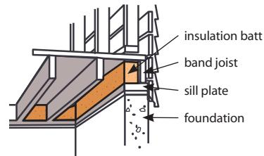
Cut insulation to fit band joist spaces between the sill and subfloor.
