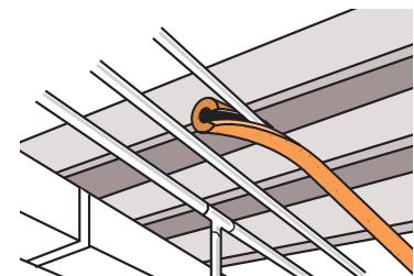
Use foam insulation on hot water pipes in your basement or crawl space. The water will stay warmer in the pipes, cutting the time you need to wait for hot water for sinks, bathtubs or showers.
