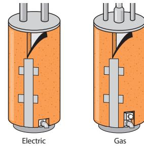
Giving your older water heater a blanket to lower your water-heating bills is an easy, do-it-yourself job. Be sure to follow the insulation manufacturer's installation instructions—the process differs for electric and gas water heaters. Note that new water heaters have adequate insulation, so their manufacturers recommend not adding an insulating blanket.
