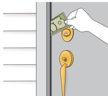
Check for air leaks in weather stripping around windows and exterior doors by closing them on a dollar bill or a strip of paper in several locations around their perimeters. If you easily can remove the bill (or it falls out), the weather stripping needs to be repaired or replaced. Also perform a visual check of every weather strip, looking for cracked, deformed or missing sections.
