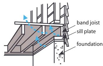
Get rid of drafts on the main floor by caulking along the sill plate and band joist in the basement.
